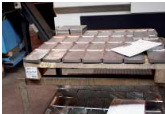
Fig. 7 Finished tamper shoes ready to install in the tamper.
